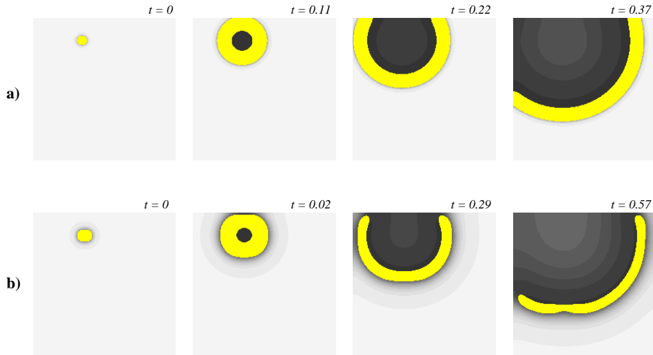
Fig. 8. Propagation of waves in the Gray-Scott model. Results of the numerical solution of equations (11) and (12) with (a) \epsilon = 0.2 , \alpha = 0.05 , and A = 1.5 ; (b) \epsilon = 0.1 , \alpha = 0.05 , A = 1.5 . In (a) the system is 10 \times 10 ; in (b) the system is 5 \times 5 . The shades of gray show the distribution of \eta . The spots show the regions where \theta > 10 .
